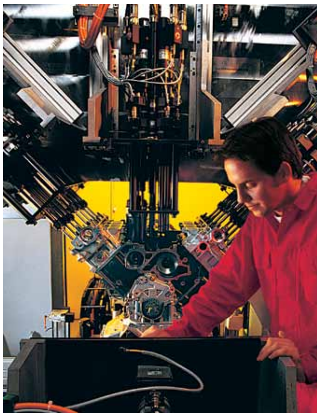
An automatic station on an engine assembly line uses two opposing electric power heads, each having 8 spindles, and a center power head of 6 spindles.
