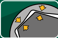
Sockets feature off-corner loading
